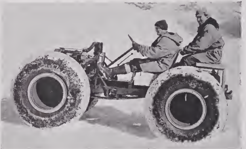
FIGURE 6. Standard 1/4-ton, 1x4 jeep equipped with 17:00x20 airplane tires.
